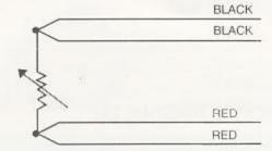
Lead configuration 3 provides two connection to each end of the sensor. This construction is used for measurements of the highest precision.
