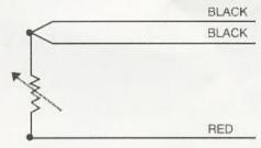
Lead configuration 2 provides one connection to one end and two to the other end of the sensor. Connected to an instrument designed to accept three wire input, compensation is achieved for lead resistance and temperature change in lead resistance. This is the most commonly used configuration.
