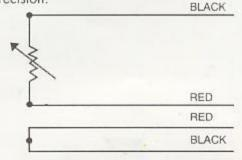
Lead configuration 4 is similar to lead configuration 3 except that a separate pair of wires is provided as a loop to provide compensation for lead resistance and ambient temperature changes in lead resistance.
